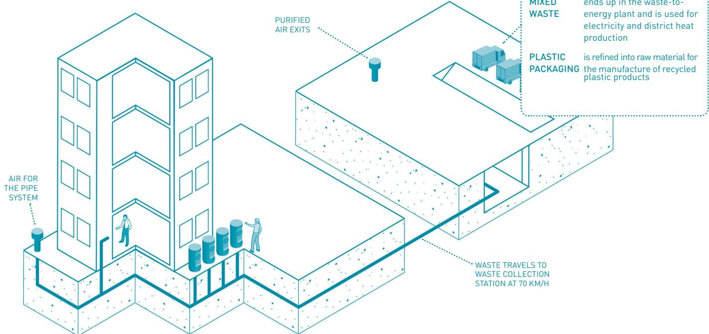
THE NEW era of residential living calls for brand new recycling solutions. At Kalasatama, there is a new, innovative pipeline-based waste collection system which introduces hi-tech into waste management on an unprecedented scale. Using an underground pipe network, waste travels to the waste collection station in a flash. Trucks gather the waste and transport it onwards – waste is utilized as recycled material, incinerated for energy or converted into biogas.
